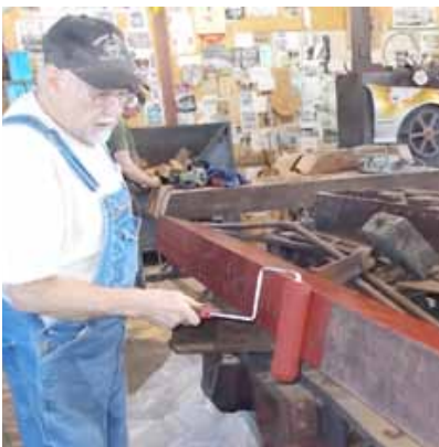
2018: Jerry paints red oxide primer on a flatcar reinforcing steel angle iron.
