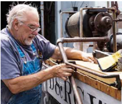
2016: Jerry installs one of eight hand holds along edge boards on the flanger.
