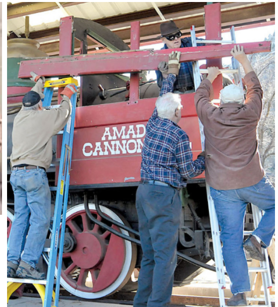
2011: Duane Danielson, Tom Artzberger, Jerry Hoffer, and Ron Nott (in cab) lift a top side rail in place on Emma Sweeny (called Amador Cannonball in Jackson, Amador County, California).
